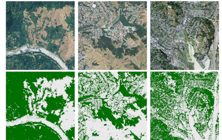
Fig 7. Classification of tree cover by boosted linear-plus-quadratic stumps, from the 508-qubit problem. Left: A region of broken tree cover outside the town of Blocksburg, CA. Middle: Saint Mary's College of California. Right: The city of Mill Valley, CA.
